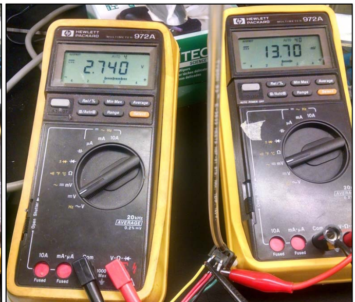
Gain set to 200 for amplifier mounted on TP2. ~1 psi load applied to pressure transducer 26PC6BF2G via vertical tube of water. (10/2014)
